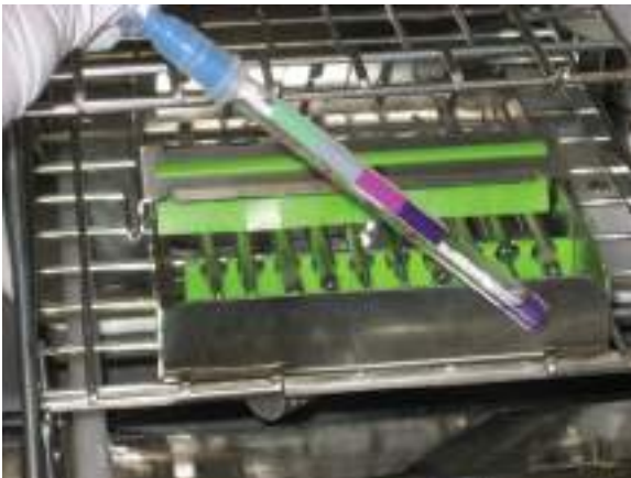
Figure 7.15 Protein detection test. (a) A random set of instruments and tray are swabbed and the swab is inserted into the test solution of ninhydrin. If protein is present the solution will turn blue-purple. (b) A pass test. (c) A fail.
