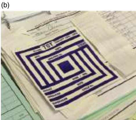
Figure 7.18 (a) A Bowie–Dick test kit showing the yellow test sheet in the centre of the paper pack. (b) A ‘pass’ Bowie–Dick steam penetration test pasted into the sterilizer logbook. (c) A ‘failed’ Bowie–Dick test indicating a failure to remove all the air from inside the test pack and replace it with steam, as demonstrated by an incomplete colour change on the indicator sheet.
