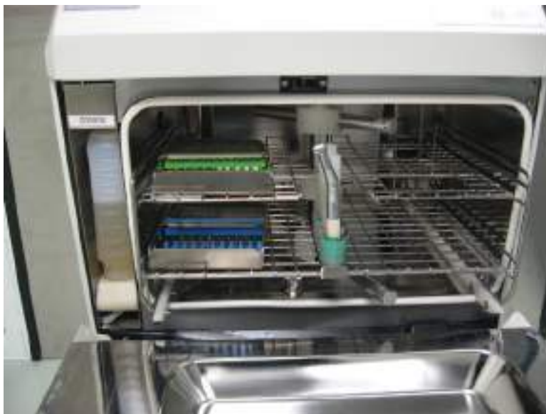
Figure 7.13 Handpiece connectors in a thermal washer disinfecter. If the connector is fitted with a filter, these require regular cleaning.
