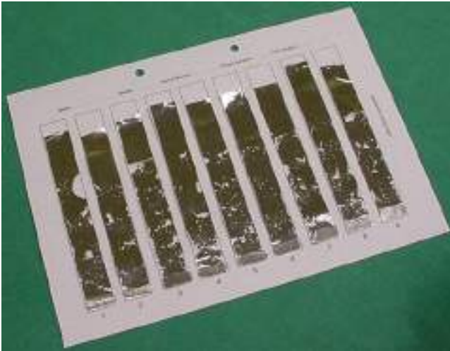
Figure 7.16 Foil ablation test. (a) Nine foil strips suspended from a 3 × 3 grid made from masking tape suspended across the ultrasonic bath. (b) Close-up view demonstrating pitting and perforation of the foil strips indicating that the ultrasonic bath is working satisfactorily. (c) Foil strips mounted on a test sheet, retained as a permanent record in the machine logbook. Source: Courtesy of Paul Jenkins.
