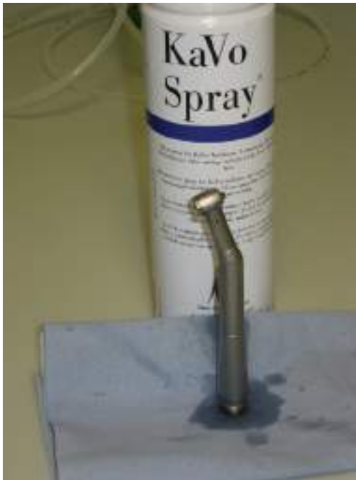
Figure 7.12 Service oil is sprayed into the handpiece and the excess oil is allowed to drain out.
