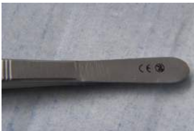
Figure 7.22 International symbol designating 'single-use only' on disposable tweezers. Note the pitting and striations of the metal surface of this single-use item, which would impede any attempts at resterilization.
