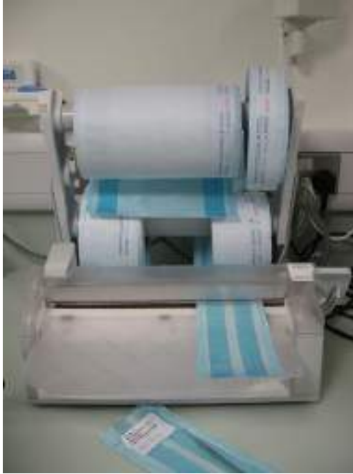
Figure 7.8 Heat sealing machine in the clean zone to seal instrument packs either before or after sterilization. The machine is fitted with rolls of packaging of different sizes suitable for use with a range of trays sizes or for packing single instruments.
