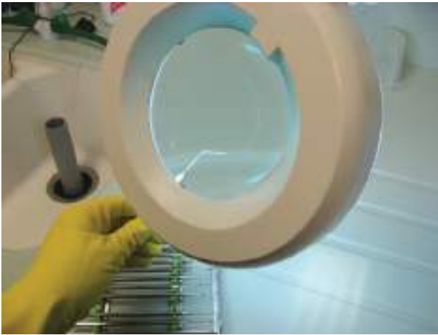
Figure 7.9 Manual cleaning of instruments. (a) Keep instruments immersed during cleaning. Note the use of a standpipe plug, which acts as an overflow as instrument washing sinks like hand basins are constructed without overflows. (b) Inspecting an instrument for residual debris or rust spots using an illuminated magnifier. Dispose of rusted instruments.
