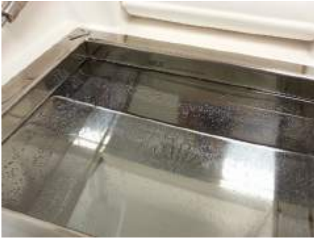
Figure 7.14 The figure shows bubbles of dissolved oxygen in an ultrasonic bath. If not removed, they collect on the surface of the instruments and interfere with the cavitation action of the bath. They are removed by degassing the bath.
